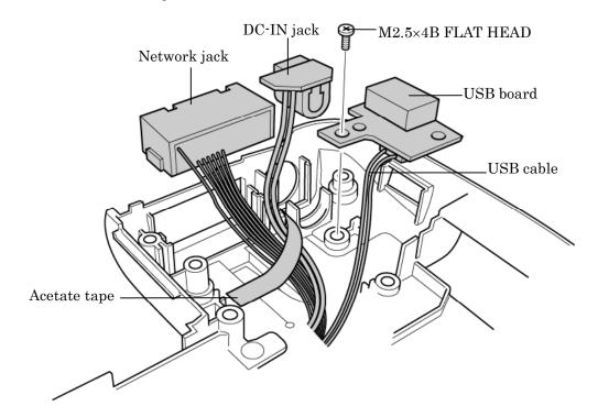
Figure 4-34 Removing the USB board/DC-IN jack/network jack
